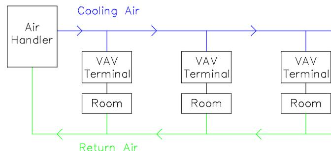
The air handler uses a fan to circulate warm air returned from the rooms through a cooling coil and back to the rooms through the air ducts and VAV terminals. Air handlers include dampers and controls to regulate the mixing of fresh, outside air with the returned air, and controls to regulate the cooling air temperature.
