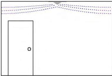
As the air stream travels away from the diffuser, it continues to take in surrounding air. The air stream slows down and moves away from the ceiling. This action mixed the cooling air with warm air, so the temperature is much closer to the actual room temperature. This air drops toward the bottom of the room in a broad, gentle pattern. Adequate diffuser velocity produces proper air distribution and a proper temperature envelope.
