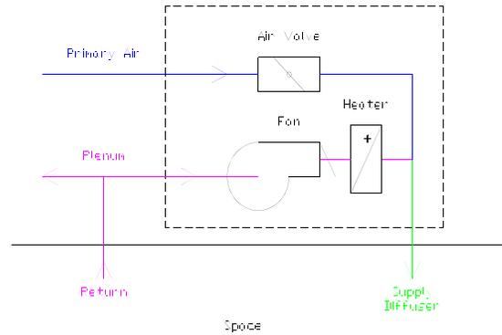
The parallel fan turns on when the cooling volume falls below the level required for the diffuser to function. The fan turns on, increasing the diffuser velocity. Cooling air mixes with air from the fan, and the diffusers distribute it evenly throughout the conditioned space. When the fan is off, a back draft damper prevents cooling air from flowing backward through the fan.
