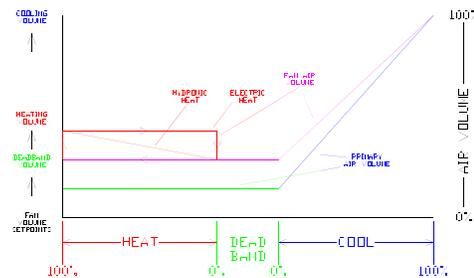
If electric terminal heat is used, the fan speeds up to the heating volume when the heating element is on. When the heating element turns off, the terminal fan slows to a lower volume.
