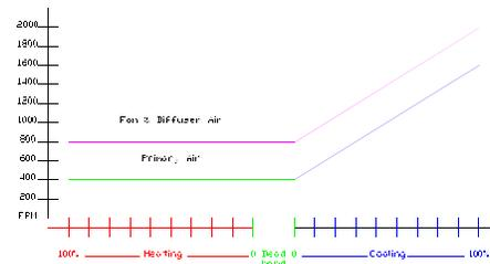
Low temperature systems allow reduction in central fan size and may also be used with ice storage systems. In these applications, the series terminal mixes warm plenum air with low temperature cooling air to prevent low temperature discharge from the diffuser.
