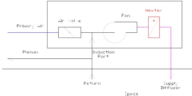
The series fan attempts to deliver a constant air volume to the supply diffusers. It draws air from the outlet of the air valve, or from the induction port to maintain this air volume.
